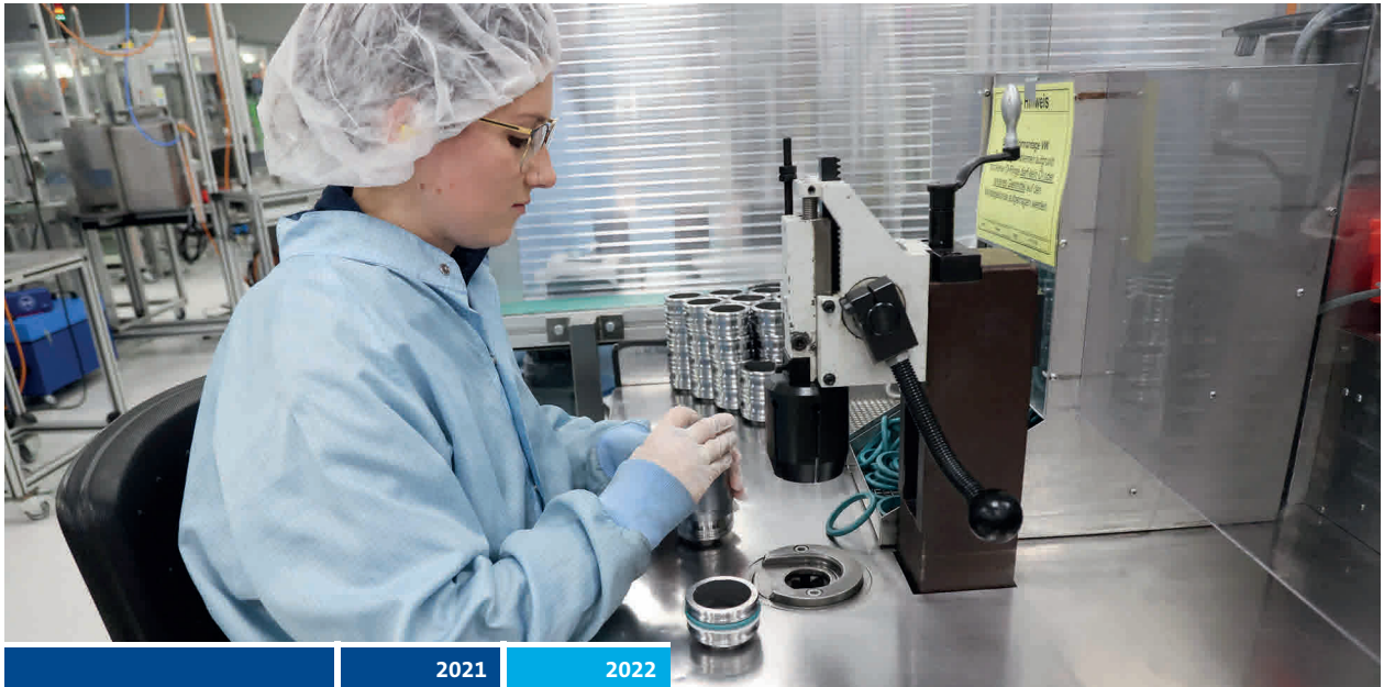
Seal assembly in the clean room for accumulator production at Freudenberg Sealing Technologies in Remagen
