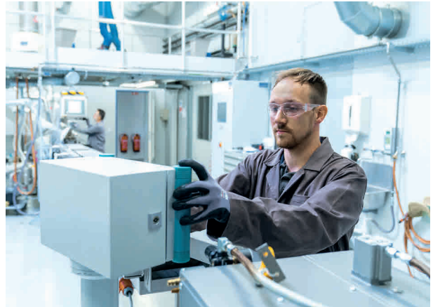
A Freudenberg employee preparing polymer materials with a twin-screw extruder.
