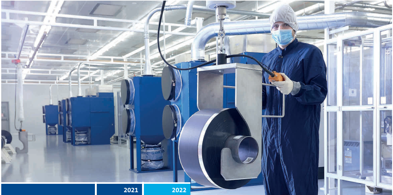
An employee operating a rolling unit for aluminum foil at a stamping machine – this foil is used in lithium-ion batteries.
